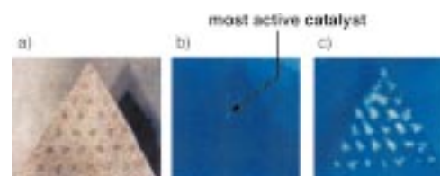
Figure 16. A ternary Pt-Rh-Os array in 6 M aqueous methanol (pH 6) with a quinine indicator. a) Image in white light. b) Fluorescence image at low overpotential, which identifies the most catalytically active region. c) Fluorescence image at high overpotential, where methanol oxidation occurs at every spot in the array. (Reprinted with permission from the author. [185] © 1998 American Association for the Advancement of Science.)
